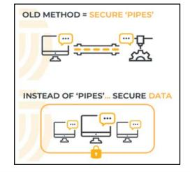
Named data networking (NDN) is a new internet architecture that enables secure end-to-end communications without depending on the security or topology of underlying channels.
