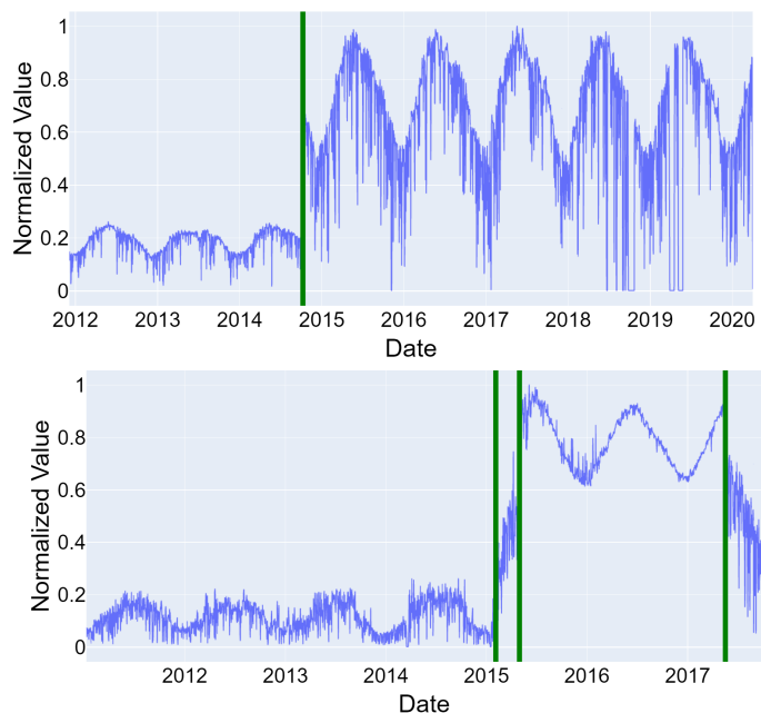
Fig. 1. Two example daily time series with data shifts, taken from data streams in the NREL PV Fleets project. Daily data points are represented in purple, and vertical green lines represent manually labeled changepoints.
