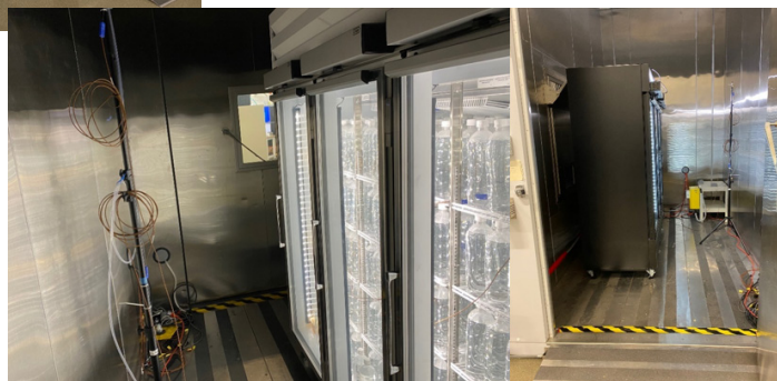
Refrigerator cases inside environmental chamber: Baseline (left), EE Case A (right)
