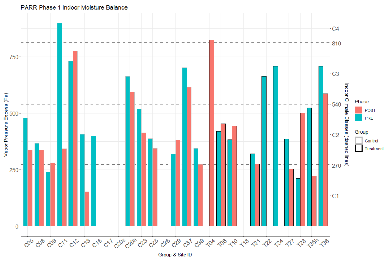
Figure 10. Phase 1 indoor moisture balance for control and treatment homes
