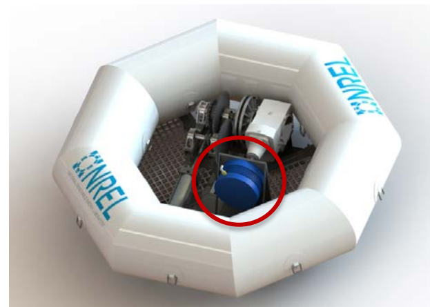
CAD model of NREL's HERO WEC with electrical generator component (circled in red). Model from Scott Jenne, NREL.
