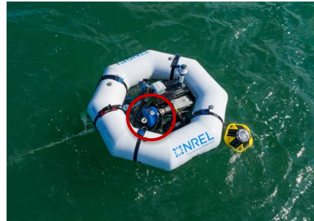
In-water deployment of NREL's HERO WEC with electrical generator component (circled in red). Image by John McCord, CSI.
