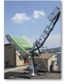
Used to accelerate material degradation by exposure to concentrated UV light.<sup>1</sup> R&D100 winner
