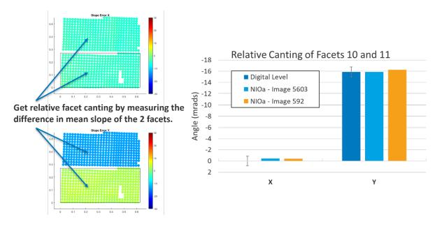
**Figure 9**. Left: The relative canting of adjacent facets is measured by comparing average measured slopes. Right: Two ReTNA results are compared to a high-precision digital level measurement.
