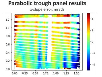
**Figure 7**. ReTNA results for slope error in the x-direction on a parabolic trough mirror.
