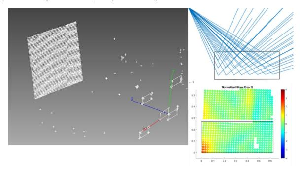
**Figure 5**. Photogrammetry is used to create a 3D scene (left). Once the camera point is solved, the mirror's surface slope can be measured (top right) to yield ReTNA results (bottom right).
