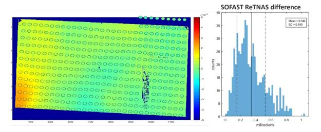
**Figure 8.** Left: ReTNA slope errors in the x direction (circles) are plotted directly on top of the same measurements from SOFAST (background). ReTNA and SOFAST results are plotted on the same color scale, showing good agreement. Right: ReTNA point values are subtracted from the SOFAST measurements to produce a difference distribution.
