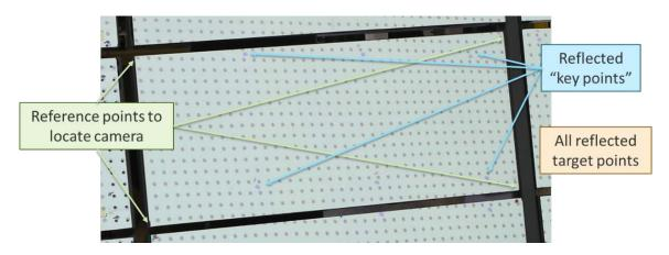
**Figure 4**. An expanded image of targets reflected in a mirror facet. Mirror corners, reflected target points, and reflected coded key points are identified for analysis.
