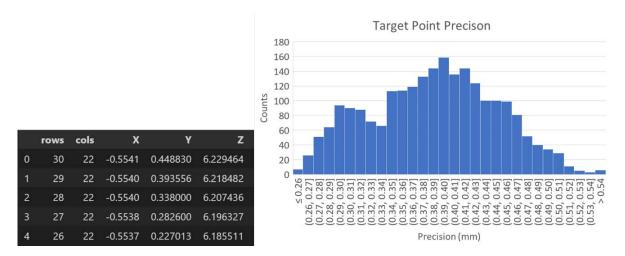
**Figure 2**. Photogrammetry is used to generate a library of target point locations (left). The precision of each target point is plotted (right).
