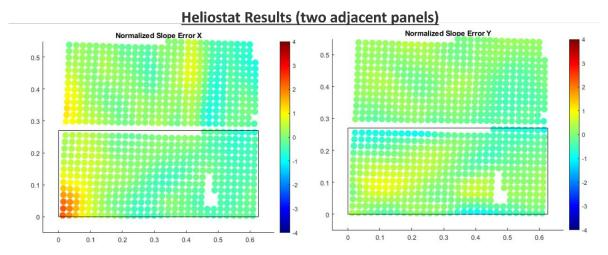
**Figure 6**. ReTNA results on adjacent heliostat facets in the x-direction (left) and y-direction (right).
