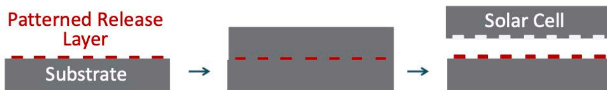
Figure 24 (Left) A substrate with a patterned mask. (Middle) An epilayer produced by nucleation, lateral overgrowth, then coalescence. (Right) Substrate separation from the epilayer at the weakened layer. For substrate reuse, the process is repeated.
