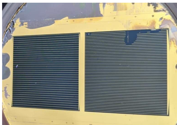
Figure 7. (left) Subcell JV curves of large area ( 4 \text{ cm}^2 ) 4T GaAs/glass/Si IBC tandem solar cells. (right) Photo of two 4 \text{ cm}^2 GaAs subcells processed on a 4 inch wafer grown at SolAero.
