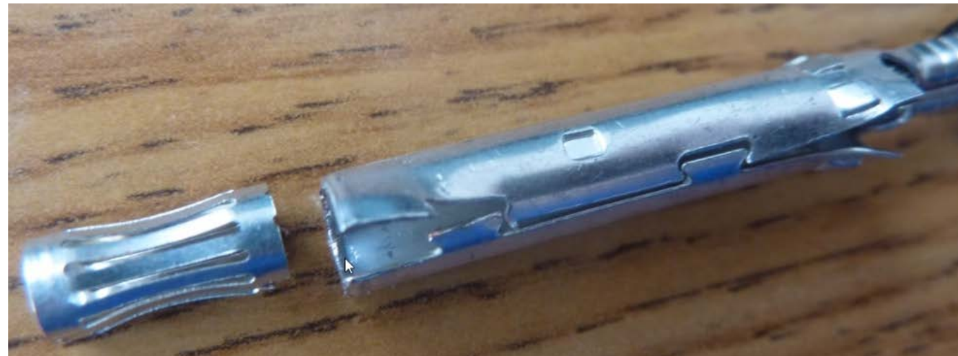
convolute spring, extracted from unaged metal pin
