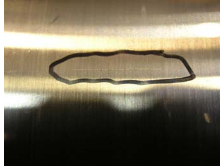
Axial cracks (gearbox bearings)
