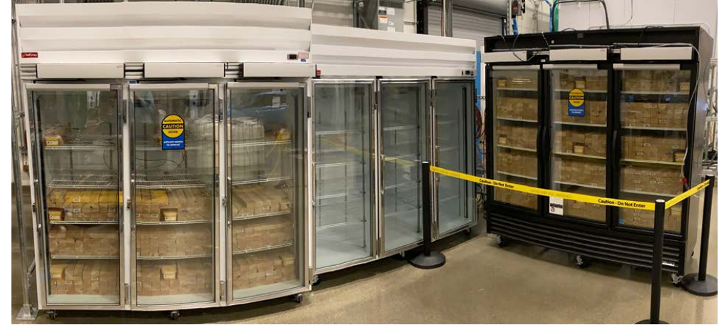
R134a (Left), R513a (Center): Howard McCray (HMC) Model GR75 R290 (Right): True Manufacturing Model GDM-72-HC~TSL01
