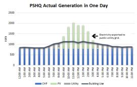
The second microgrid installed at the corrections facility includes a 240-kilowatt CHP system added to the existing diesel generators. This system decreases annual greenhouse gas emissions by an estimated 950 metric tons due to the CHP technology, compared to present-day grid-supplied energy and onsite diesel generation. (Walker, 2021)
