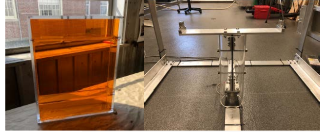
FIGURE 3 – OSWEC scaled model. (Left) OSWEC fabricated mode. (Right) Foundational tube assembly with the six-axis load cell installed at the base.
