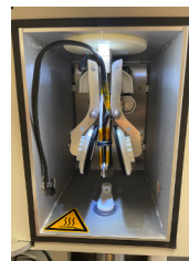
Fig. 3: Biasing sample holder in Vitrobot.
