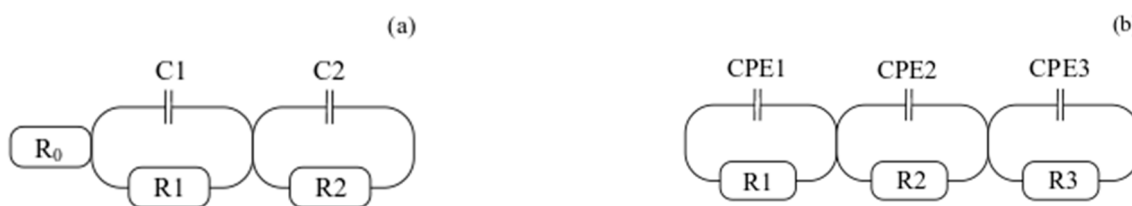
Figure 10. Equivalent circuit models chosen for a DMFC cathode, with a series connection of an ohmic resistance and two R-C combinations representing a Faradaic impedance (a), with a series connection of three R-CPE elements, representing the ORR, methanol oxidation and mass transport limitations (b).
