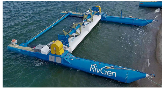
FIGURE 3: ORPC RIVGEN POWER SYSTEM [6]
