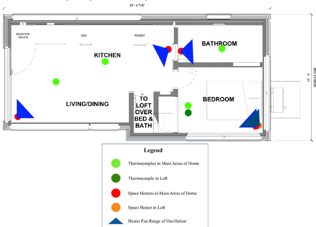
Figure 8. Layout of sensors and space heaters in the test home
