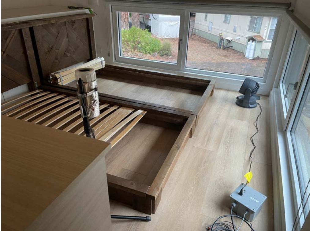
Figure 13. Space heater, controller/watt node, and aspirated thermocouple in the loft
