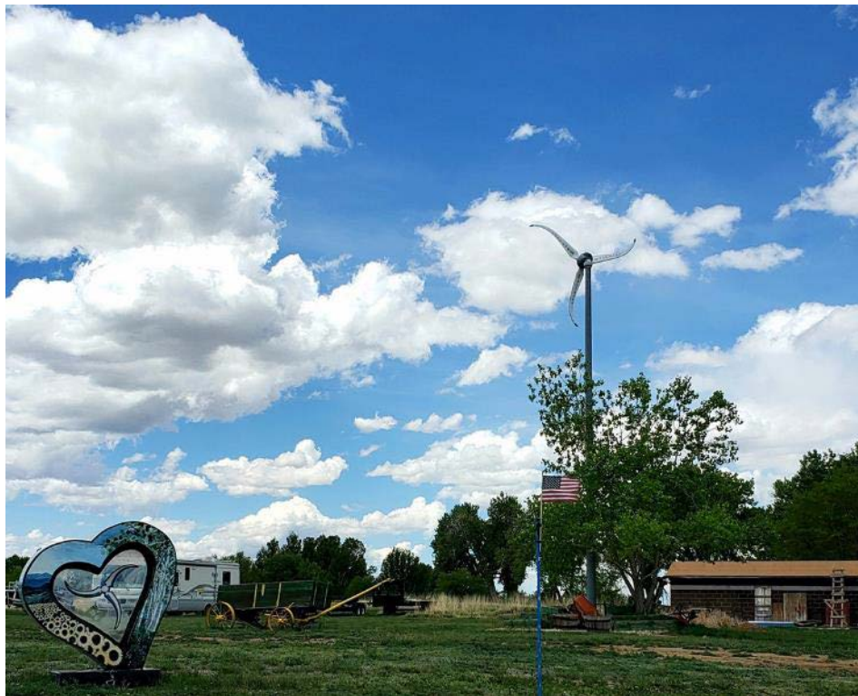
Downwind passive yaw Skystream turbine. Photo from PNNL Distributed Wind Photo Gallery
