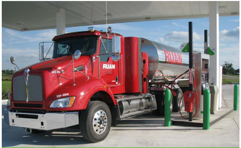
A Ruan milk transport truck fuels up at an ampCNG renewable natural gas (RNG) station in Indiana. The RNG is produced from cow manure—from the same cows that produce the milk. Photo from ampCNG, NREL 37376
