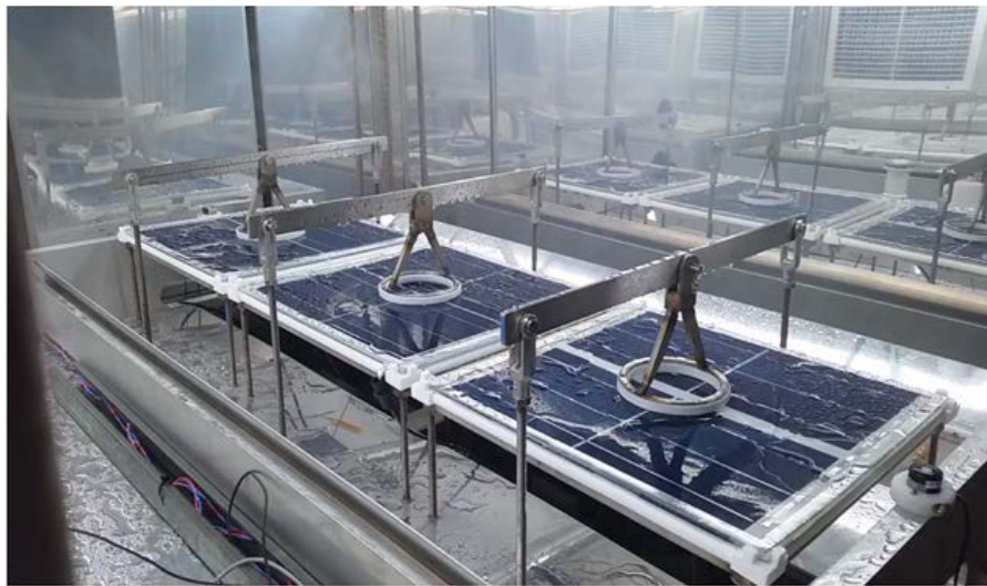
Figure 6: Modules under test inside the C-AST chamber.
