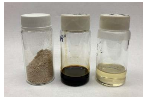
Image: poplar ( left ), lignin oil ( middle ), lignin-derived SAF blendstock ( right )
