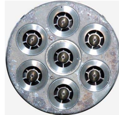
The 7 swirler in the test rig (ALF)
