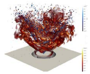
Simulation of SAF in swirled liquid fuelled burner, SNL 2022 (Image courtesy: Landon Owen, Bruno Soriano SNL)
