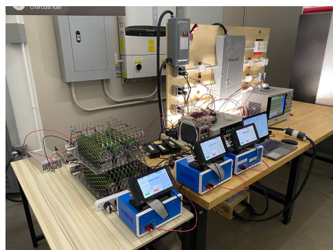
Figure 16. Testbed hardware with power analyzer, laptop, LEDs and resistive load banks. (Photo used with permission by Arthur Santos of Colorado State University.)
