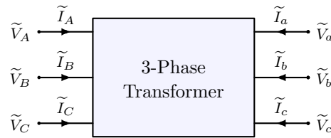
Figure 7. Three-phase transformer component.
