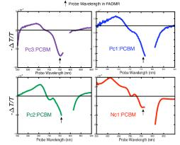
Photoinduced absorption (PA) spectra (above) show *electronic* state absorption under steady-state excitation conditions. For PADMR, the probe is set to the ground state (G.S.) and modulated RF is introduced. This allows us to measure MR effects on charge and/or exciton *recombination* dynamics.
