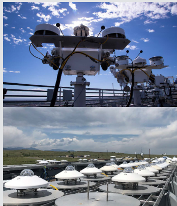
Figure 1. Radiometers deployed at NREL and ready for BORCAL calibration. Photos by Afshin Andreas, NREL
