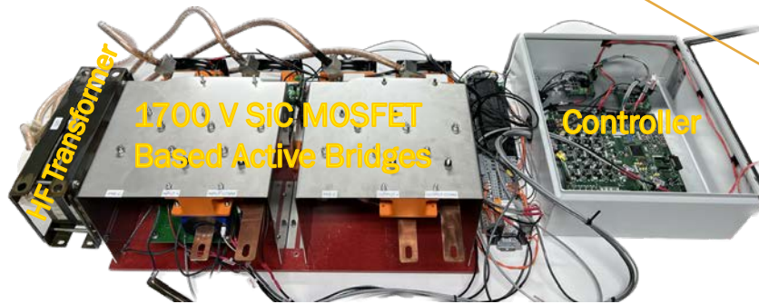
1000 V, 175 kW, 20 kHz DC/DC Charger 34" x 20" x 15"
