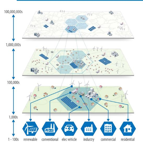
Autonomous Energy Systems (AES) aim to use cutting-edge optimization algorithms and hierarchical, distributed control architectures to
