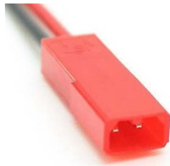
Figure A-13. Team-provided connection to the manual shutdown interface. Image created by Lee Jay Fingersh, NREL
