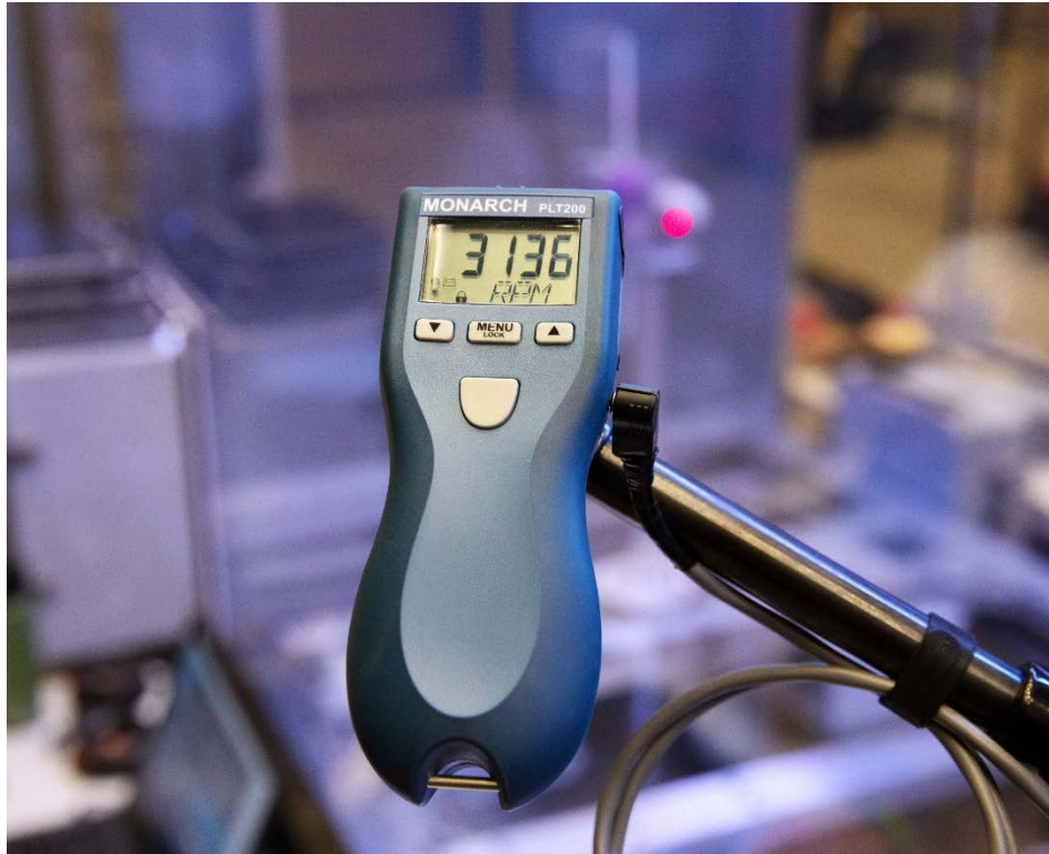
Figure A-15. Laser tachometer used to measure turbine revolutions per minute. Photo by Werner Slocum, NREL
