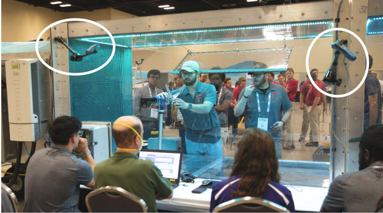
Figure A-16. Laser tachometer sensors (circled in white) used to measure wind turbine rpm. Photo by Werner Slocum, NREL
