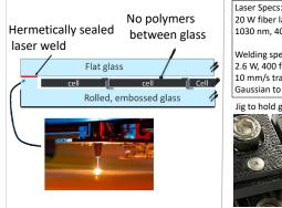
20 W fiber lase 1030 nm, 400 fs – 200 ps pulse Welding specs: 2.6 W, 400 fs pulse, 200 Hz 10 mm/s translation
