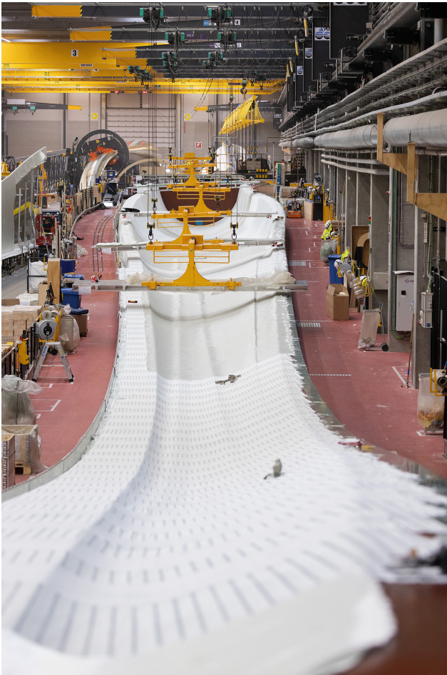
Figure 13. Most wind turbine blades are manufactured as two shells, each with an embedded spar cap. The two shells are connected with shear webs forming the internal structure. This 97 m long blade from Siemens Gamesa has a continuous fiber reinforced composite skin and spar cap running all the way from the circular root, where it attaches to a pitch bearing, to the carefully designed low-noise tip (foreground). (Photo credit: Siemens Gamesa Renewable Energy.)
