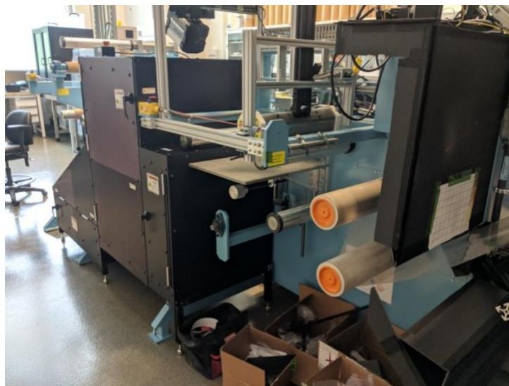
Figure 1: The NREL “metrology” roll-to-roll was selected as the appropriate tool for integration of the multiplexed laser ablation web processing.
