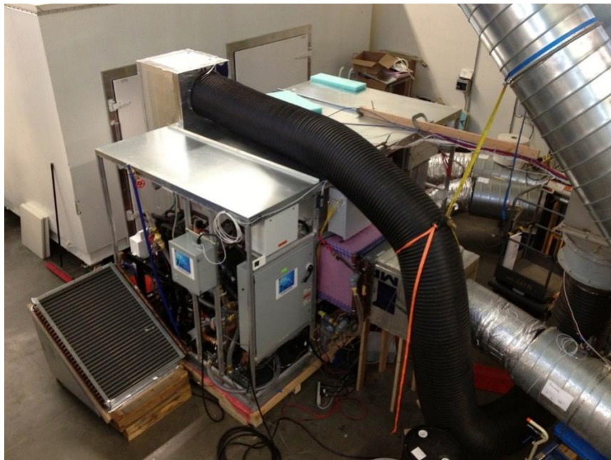
Figure 12. Prototype 10-ton system evaluated at NREL's HVAC facility in Golden, CO. The prototype system, not intended to be installed in the field, was used to characterize the combined refrigeration and liquid desiccant heat exchangers together to understand performance and design trade-offs.
