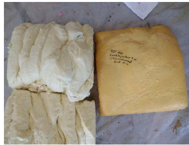
Figure 64. Pour foam compared to froth foam
