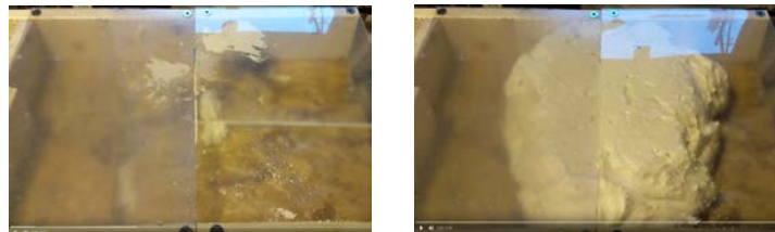
Figure 22. Perpendicular tube shot in uninsulated cavity
