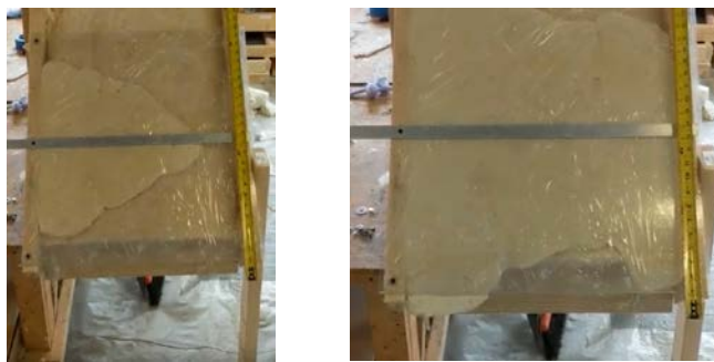
Figure 29. Top plate cross cavity in under-insulated cavity
