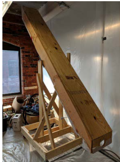
Figure 9. Length dispense test stand: angle iron pivot in center, soffit at bottom right, ridge at upper left
