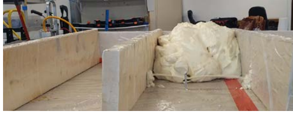
Figure 60. Single needle shooting sideways in narrow open cavity
