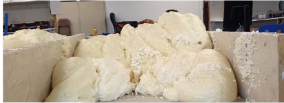
Figure 61. Dual needle shooting next to rafter in wide open cavity
