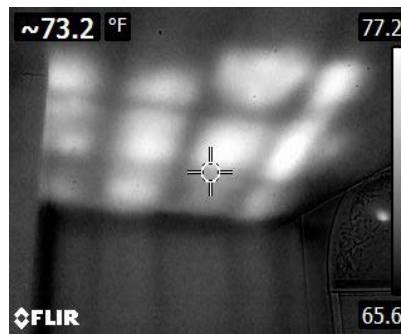
Figure 39. IR image of injected ERC
