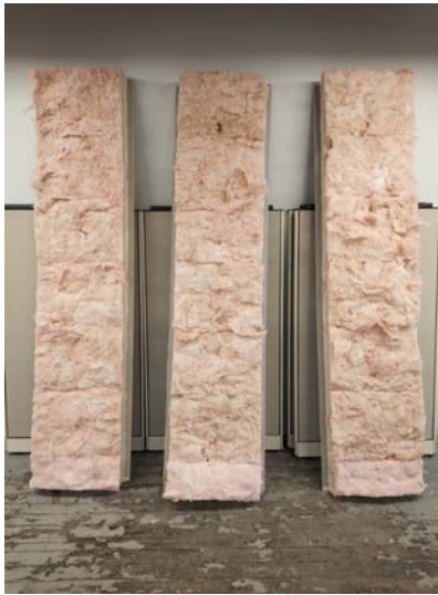
Figure 14. Foam blocks with fiberglass attached used for E84 fire testing
