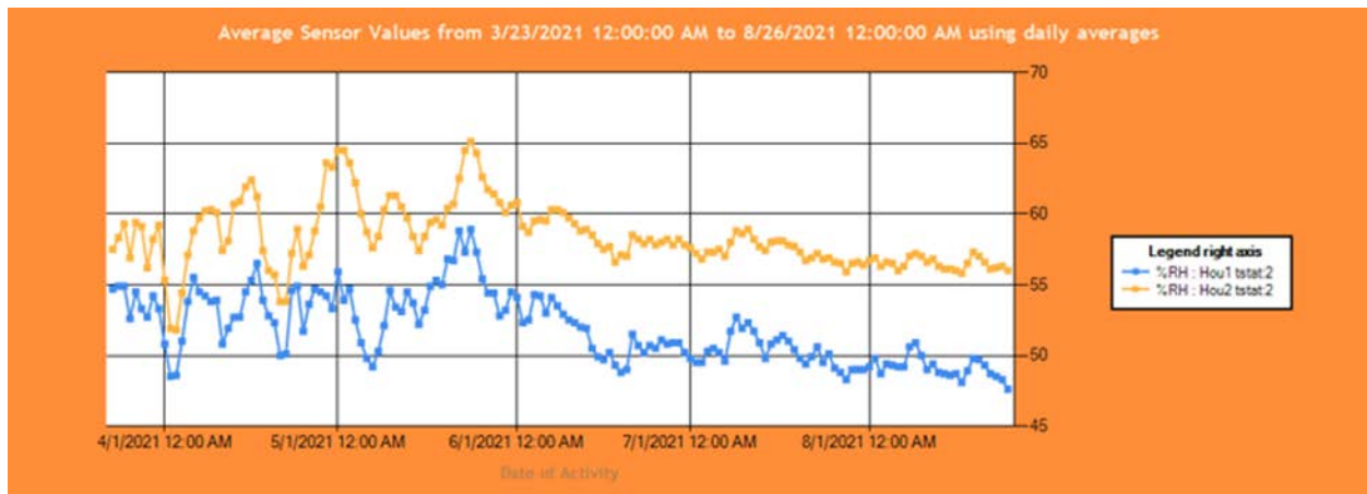
Figure 12. Houston indoor RH: test house (blue); baseline house (gold); daily averages Mar 23–Aug 26, 2021
