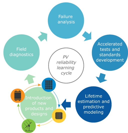
Fig. 19. PV reliability learning cycle, enabling continuous improvement to ensure quality despite ongoing technological changes.
