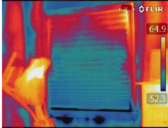
Figure 21. House 3 interior infrared image of bedroom window
