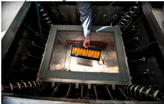
Top view of large calorimeter test chamber
