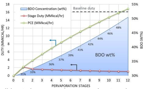
The use of pervaporation on dilute BDO concentration stream did not show superior energy/cost savings compared to the SOT evaporation/distillation.
