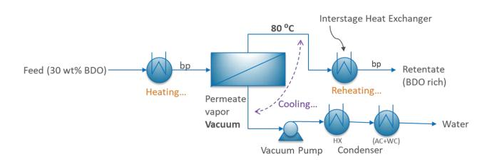
The use of pervaporation on dilute BDO concentration stream did not show superior energy/cost savings compared to the SOT evaporation/distillation.
