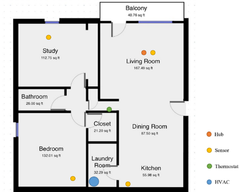
Figure 12. Floorplan and system installation
