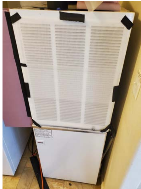
Figure 137. Photo of evaporator fouling simulation
