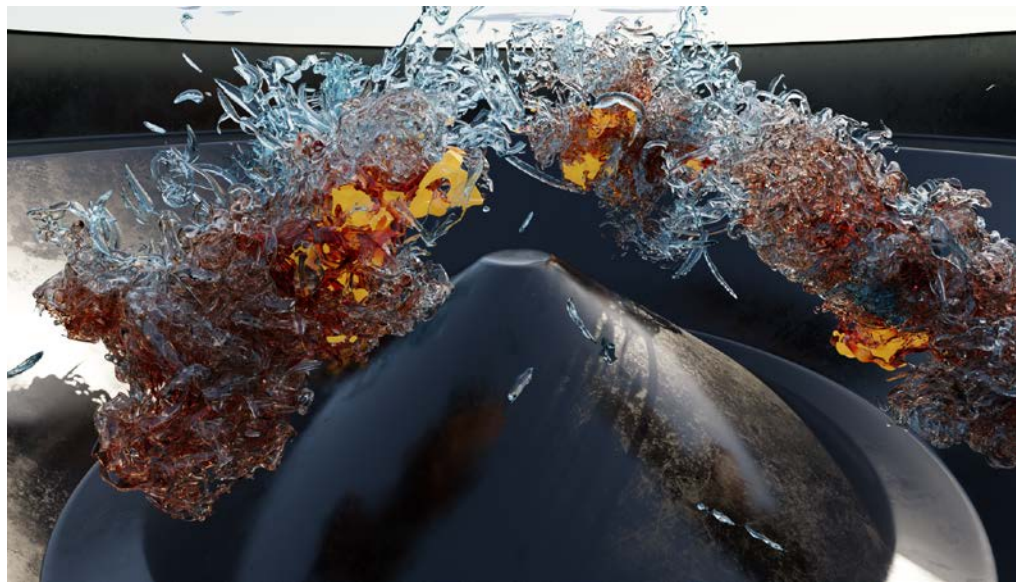
Ignition of n-dodecane jets in a closed cylinder at 60bar, computed with PeleLMex on Frontier
