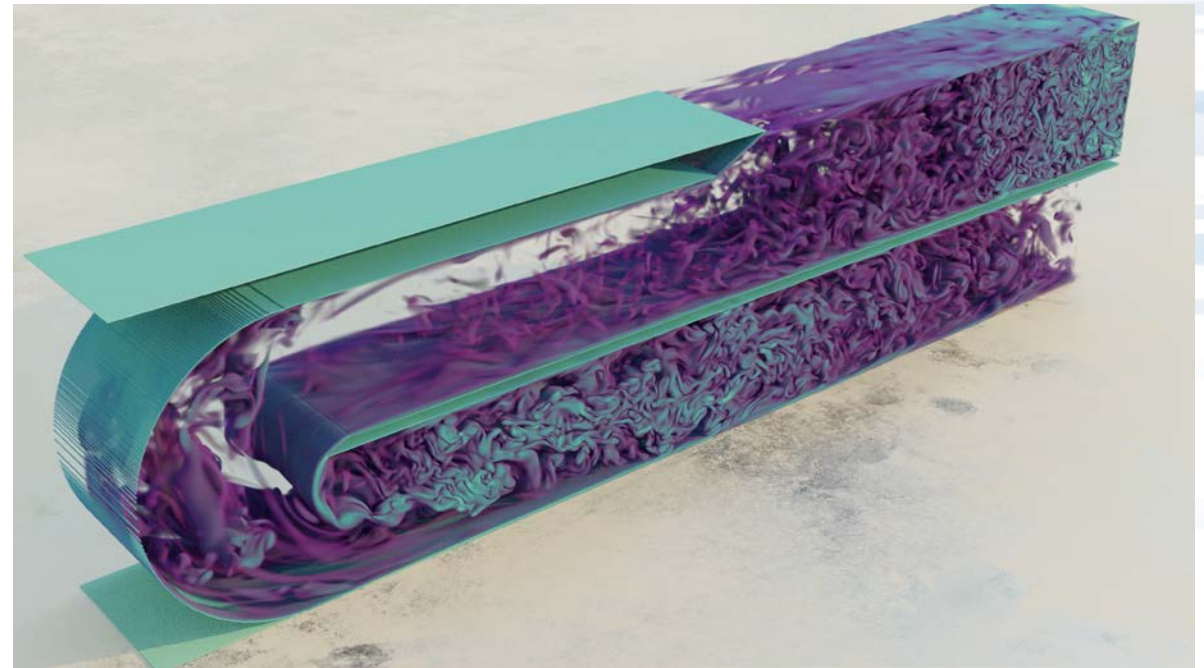
Advanced fuel nozzle simulations using PeleC for high H 2 -CH 4 fuel blends to avoid flashback in stationary gas turbines
