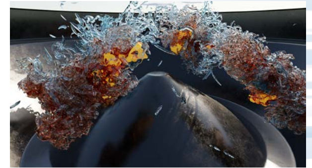
Compression ignition in a high-pressure combustion chamber, computed on Frontier as part of Exascale Computing Program Challenge Problem, 2023
