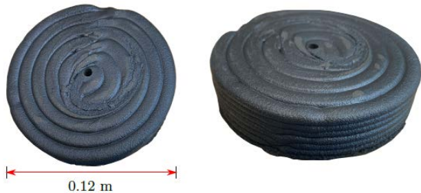
Raw samples of an AM 75 vol% NdFeB-SmFeN magnet used to measure B-H curves.
