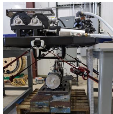
Fig. 5. Image of the laboratory test setup that was built to verify system operation of the HERO WEC (image credit: Scott Jenne, NREL)
