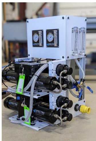
Fig. 4. A picture of the RO system that was deployed in North Carolina, USA, in 2022 (image credit: Scott Jenne, NREL)
