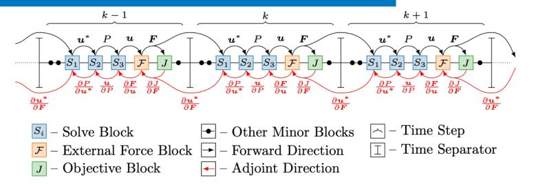
A depiction of how dolfin-adjoint records the forward problem and objective function on to a tape. Then using the reverse process to propagate the gradient backwards through this tape.
