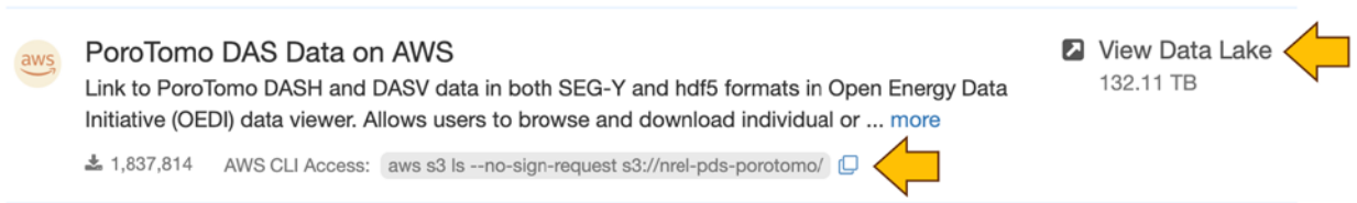
Figure 5 Screenshot of a data lake resource with links to browse the data through the data lake viewer (top arrow) and to copy the code for direct command line access to the data (bottom arrow)
