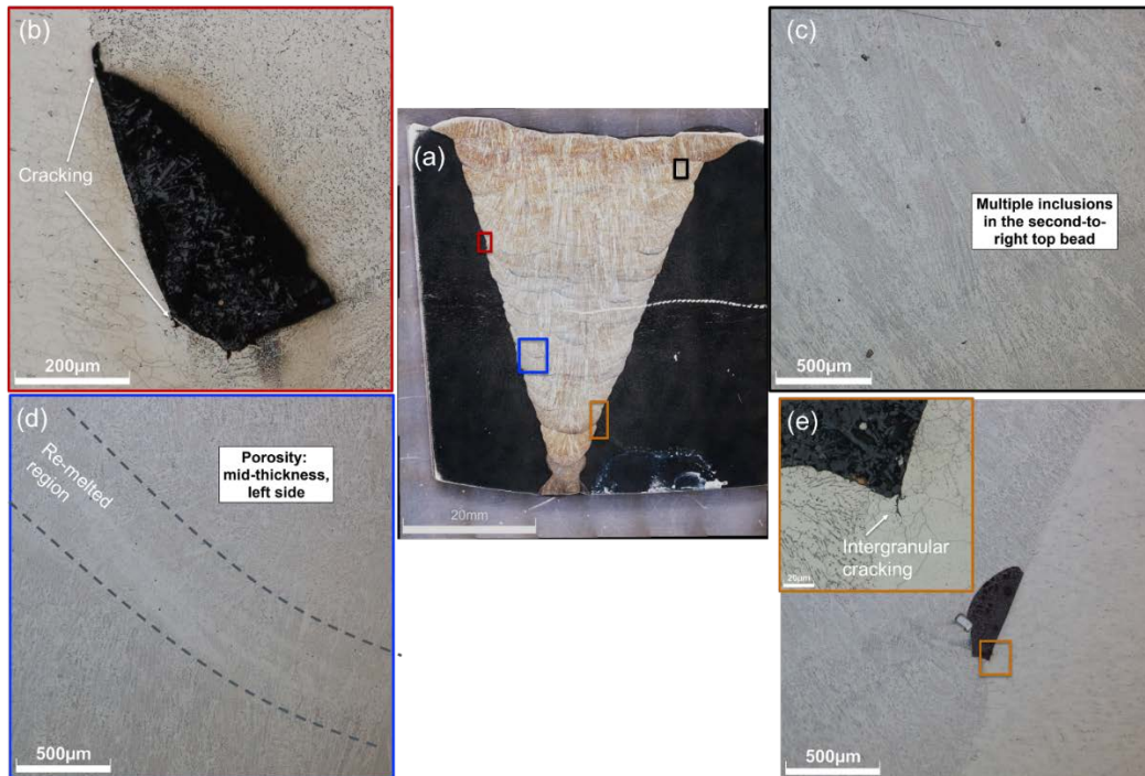
Figure 61. Weld defects in 2” thick 40 pass lab weld. Images taken after PWHT and NDE. (a) macro cross section, (b) slag inclusion and lack of fusion-indication #12 with length of 588µm, (c) smaller slag inclusions in upper right corner of weld, (d) appreciable porosity in re-melted region in the lower left half of the weld, and (e) slag inclusion and lack of fusion in lower right corner of weld with intergranular cracking initiation
