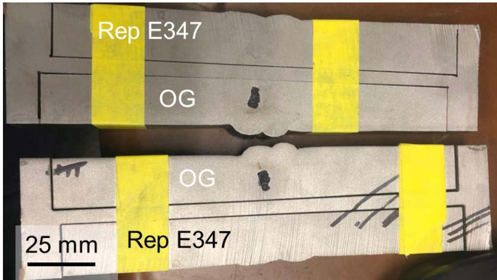
Figure 86. 8x5 mm slag inclusion/lack of fusion defect observed on side used for the intended OG samples. The defect extended to three 0.5” wide samples, indicating a 1-1.5” long defect along the weld direction. This was observed near the intersection and thickness transition between the seam and girth weld.
