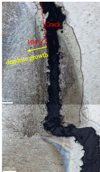
Figure 68. Second region of crack propagation into weld metal underneath OD surface with dendrite growth direction indicated
