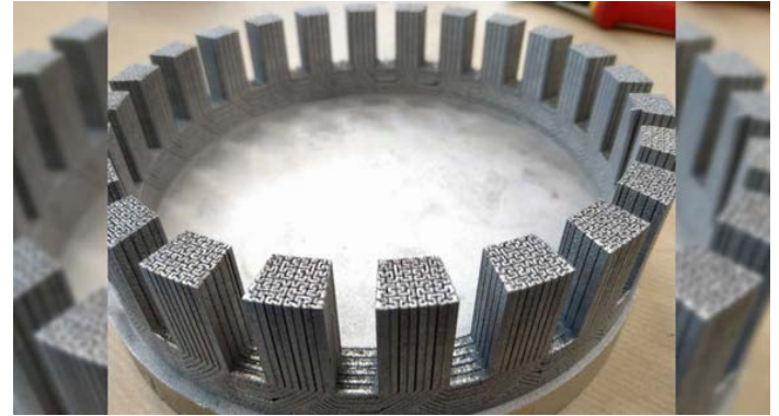
New cross-sectional geometries have been shown to reduce the eddy current losses in cores (Goodall et al. 2023).
