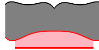
Symmetric pole: constant air-gap
