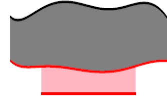
Asymmetric pole: constant air-gap
