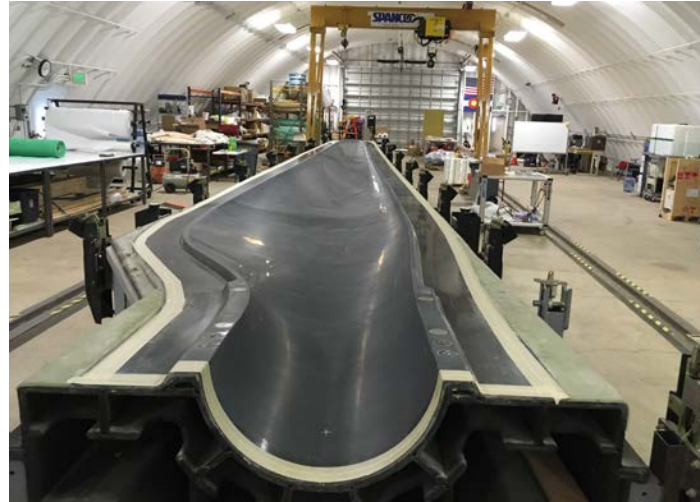
3D-printed 13-m wind blade mold. Photo by Ryan Beach, NREL
