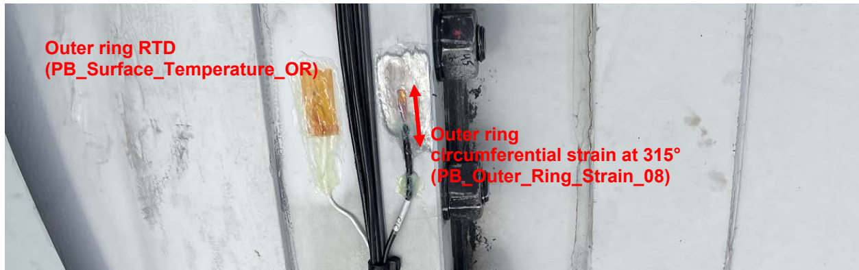
Figure 9. Outer ring temperature and circumferential strain at 315°. Photo by Jesse Graeter, ONYX Insight, NREL 85945
