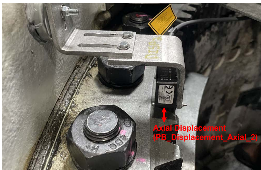
Figure 8. Relative axial displacement. Photo by Jesse Graeter, ONYX Insight, NREL 85943
