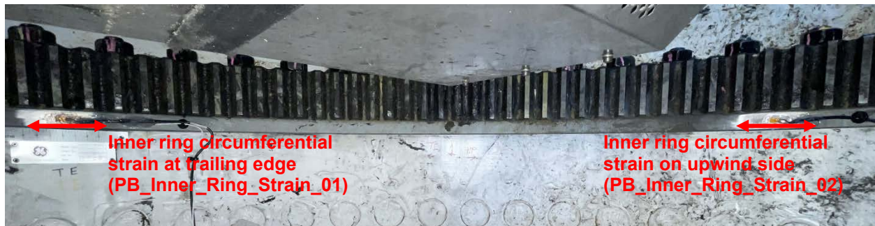
Figure 6. Inner ring strain gages. Photo by Jesse Graeter, ONYX Insight, NREL 85940
