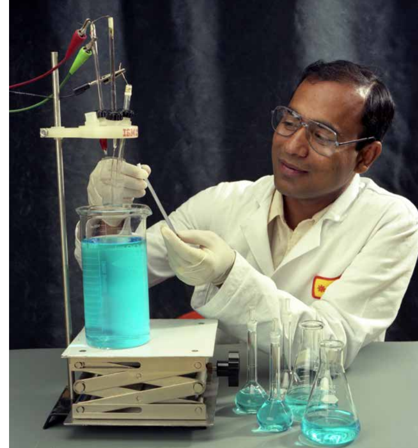
◀ SERI researcher Raghu Bhattacharya, uses a simple, yet effective electrodeposition process to coat wires, silver sheets, and nickel ribbons with superconducting thin film materials, part of SERI's foundational and applied research into new energy materials. Photo by Warren Gretz, NREL, 00075.
